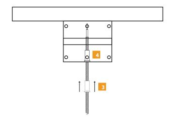
5 Push Coaxial cable all the way down until it stops.
